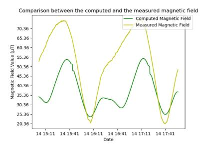
We began our results analysis comparing the measured magnetic field and the computed magnetic field. For that, we drew the graph of the magnetic field value (in  $\mu T$ ) by the time of the two data. We remarked that the shapes of the curves are globally the same, but the values differ on some places.
